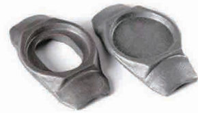
Ledger blade Material : #35Drop Forged Weight : 0.2-0.25kg Finsh : HDG, natur
